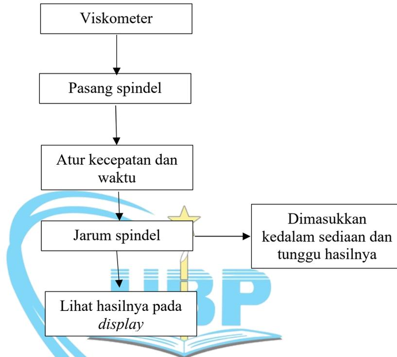
**Gambar 3.5** Diagram Alir Uji Viskositas
