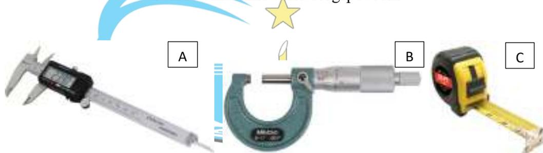
**Gambar 3.4** *Vernier Caliver* (A), *Micro Meter* (B) dan Pita Meter (C)
